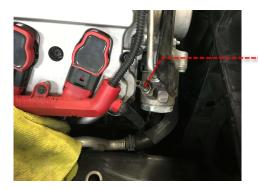
Next remove the T25 screw on the valve cover as shown, then replace it with the supplied M5x15 extension and tighten down with an 8mm socket.
