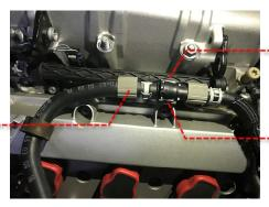
Remove the hose clamp on the end of the fuel hose using pliers and then remove the plastic coupling piece.
