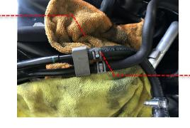
Release the fuel hose from the retaining clip, shown, and then disconnect the fuel pipe. To do this push the fuel hose into the black fixing and then squeeze the tabs on the fixing to release and then pull out.
