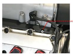
The fuel hose has a protective sleeve around a portion of it. The diagram illustrates which end to install where.
