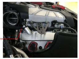
7 Install the fuel hose onto the pipe using the new fuel hose clamp provided.
