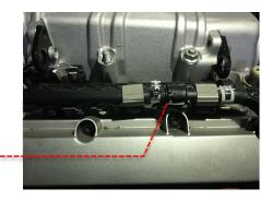
Finally, fit the other end of the fuel hose to the pipe you removed the OE part from earlier. Ensure that the hose routing is as shown in the picture, it should feed under the intake pipe and if your car has a breather hose feed it under the breather as well. Secure using the supplied fuel hose clamp ensuring that it is correctly tightened.
